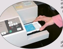
**ELISA TEST:** The enzyme-linked immunosorbent assay, or ELISA, test is particularly sensitive to high-potency medications, can be conducted rapidly, and can be read by the eye. cal diagnostic scenarios.
