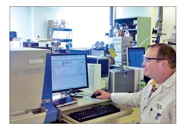
IN THE LAB: John Merchant of the Analytical and Toxicology Laboratory of the Ohio Department of Agriculture works with a thermo LTQXL liquid chromatograph-mass spectrometer (LS-MS).
